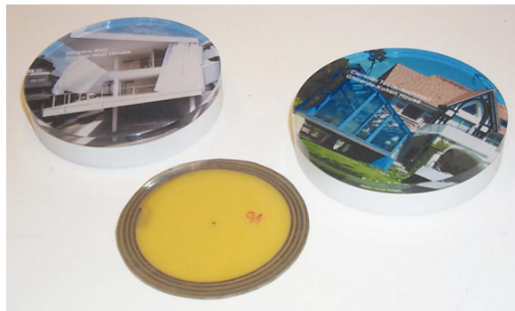
Figure 9 Photograph of the coasters with an exposed resonator in the foreground
